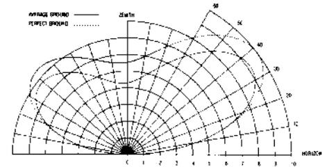
ELEVATION PATTERN (VOLTAGE) AT 6.2 MHz
