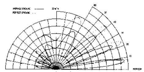
ELEVATION PATTERN (VOLTAGE) AT 30 MHz
