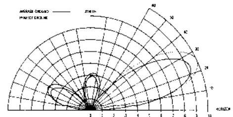
ELEVATION PATTERN (VOLTAGE) AT 9 MHz
