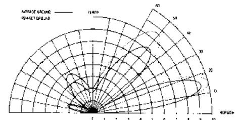
ELEVATION PATTERN (VOLTAGE) AT 15 MHz
