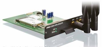
The LTE/DC-HSPA+/EDGE/GPS Module allows using all current mobile phone technologies with every stationary Viprinet Multichannel VPN Router. The newest mobile phone standard LTE – also called 4G – is already available in many countries worldwide and allows higher bandwidths and higher ranges at the same time compared to 3G. It forms the current state of the art regarding mobile phone services and thus provides long-term feasibility.
